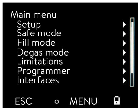
Fig. 79: Operation on the device is locked
